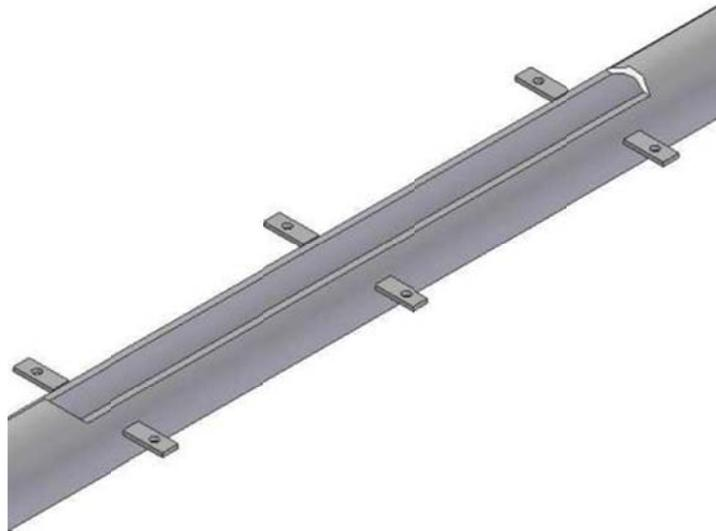
Figure 173: 4" ID stainless steel pipe with top part removed
