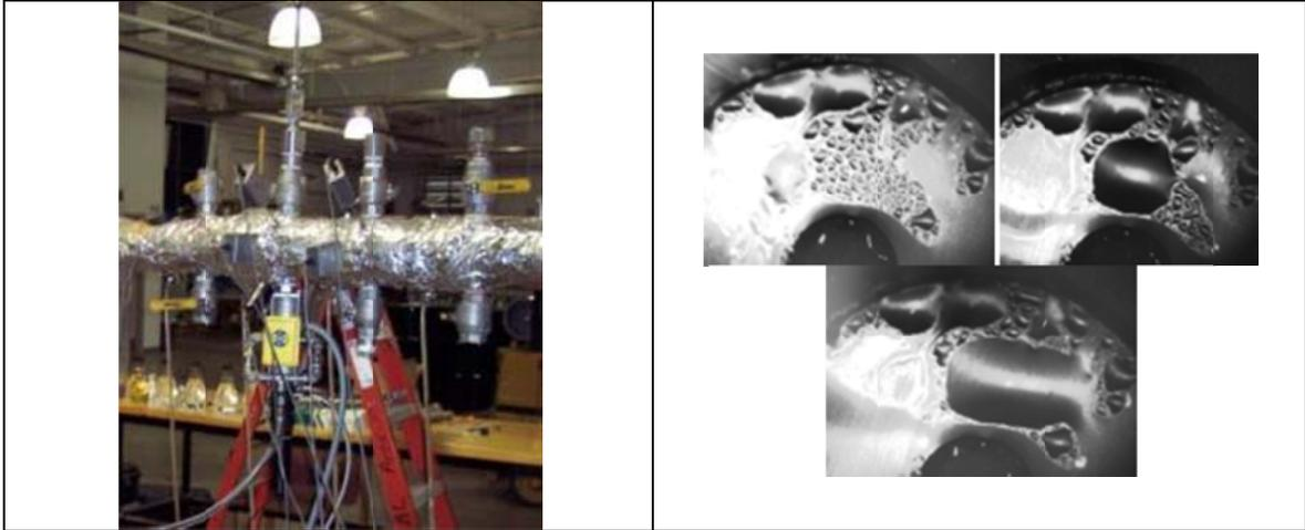
Figure 132: Test section equipped with video camera (left) – Observation of the condensation process on a weight loss sample (right)
