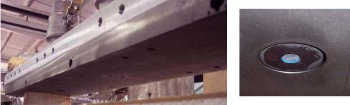
Figure 36: Stainless steel with weight loss probe ports (left) and view of the edge mismatch involved in using a flat sample in a flat slab (right)
