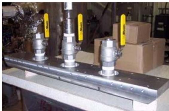
Figure 35: Stainless steel with weight loss probe ports (top view)
