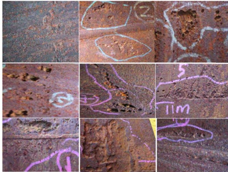
Figure 12: Typical TLC failures in  $\text{CO}_2$  dominated environment
