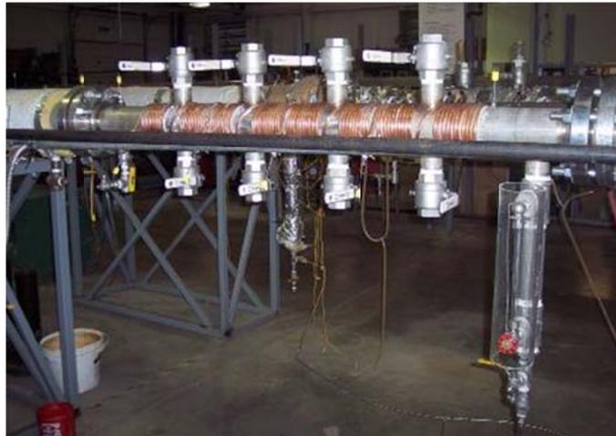
Figure 30: Typical TLC test section equipped with condensed water collector (bottom left)
