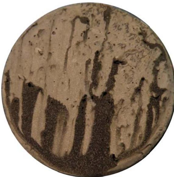
Figure 141: Weight loss sample at the end of the test
